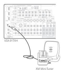
Connect an XM Mini-Tuner to the XM Radio iack on the rear of this receiver.
