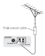
To improve AM reception, connect a 5 m to 6 m (15 ft. to 18 ft.) length of vinyl-coated wire to the **AM LOOP** terminals without disconnecting the supplied AM loop antenna.
