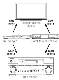
To make the most of the SR+ features, you should connect your source components (DVD player, etc.) in a slightly different way to that described in this chapter. For each component, connect the video output directly to the plasma display, and just connect the audio (analog and/ or digital) to this receiver.
