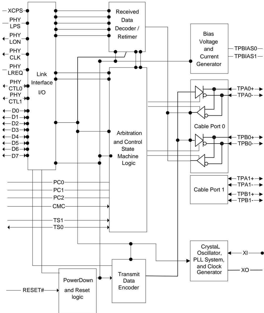
**Figure 2. Internal PHY Block Diagram**
