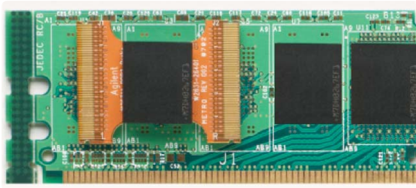
Figure 1. W2631B DDR2 x16 BGA command and data probe for logic analyzer and oscilloscope soldered onto a DDR2 DIMM
