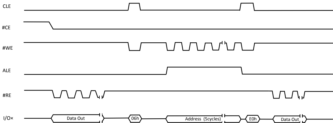
Figure 9-4 Two Plane Random Data Read (06h-E0h) Operation
