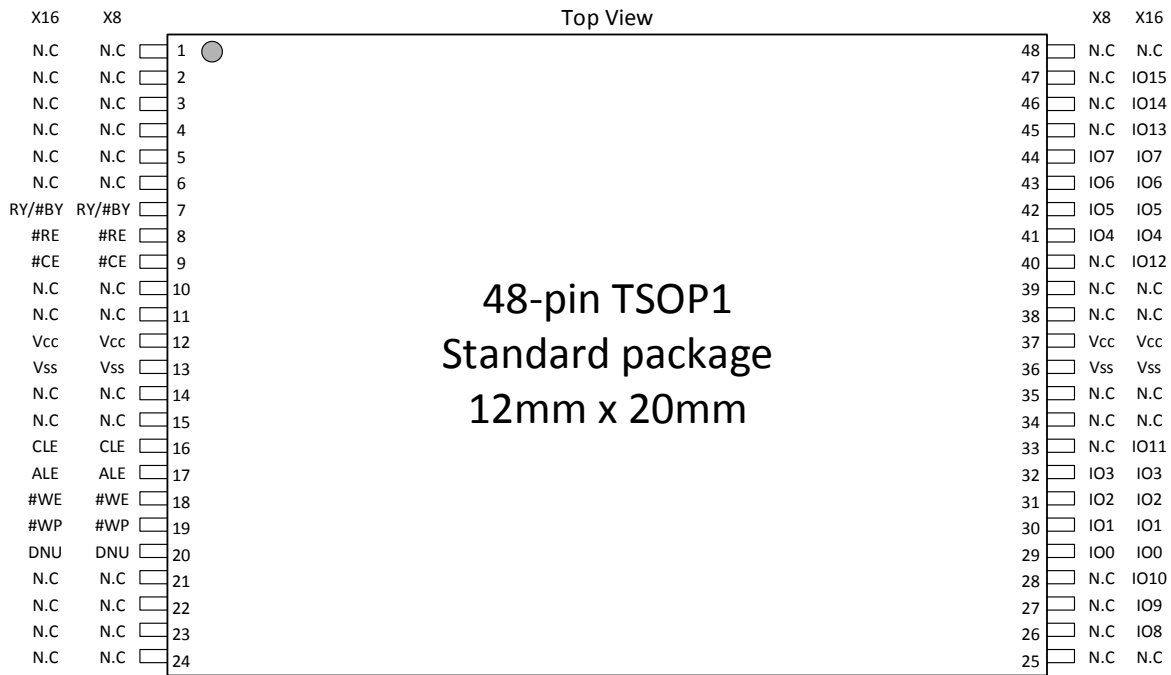
Figure 3-1 Pin Assignment 48-pin TSOP1 (Package code S)
