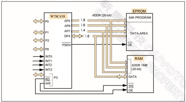
When bit 7 of the EPMA is "1," AP7<3:0> are the output pins that support memory-mapped peripheral chip select logic, which eliminates the need for glue logic. These pins are decoded by AP6<7:6>. Only one pin is active low at any time. That is, they are active individually with 16K address resolution. For example, CS0 is active low in the address range from 0000H to 3FFFH, CS1 is active low in the address range from 4000H to 7FFFH, and so forth.
