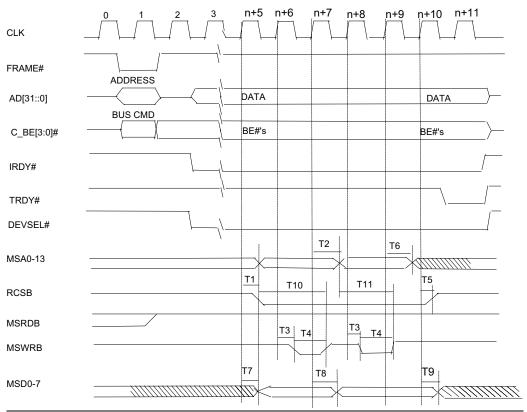
Note: 1) The other timing requirements for PCI signal are as the read transaction timing. 2) n=0,1,2,3,..... when local DMA get the control of the bus, PCI bus will insert wait state. Wait state number is n.
