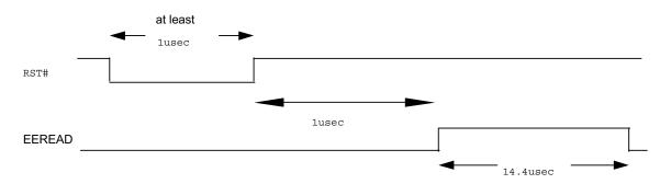
Since the ELANC-PCI reloads data into the configuration registers each time the system is reset, caution should be taken in handling resets. A system reset should keep low at least 480ns for the ELANC-PCI to decode the action as a reset. Any signal on the RESET pin shorter than this will be interpreted as noise and no response will be taken by the ELANC-PCI.
