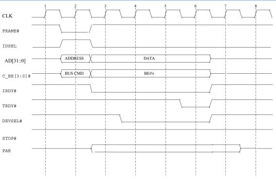
The timing is the same as the figure I/O Read Transaction, except the IDSEL is asserted during the address phase. The transaction access the configuration registers of the device.
