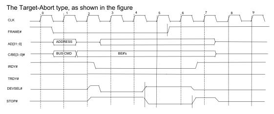
The condition is the target requires the transaction to be terminated and does not want the transaction tried again. As shown in the figure, the DEVSEL# is deasserted when STOP# is asserted. If there is a data needed to be transferred, DEVSEL# must be asserted for one or more clock cycles and TRDY# must be deasserted before target-abort can be signaled.
