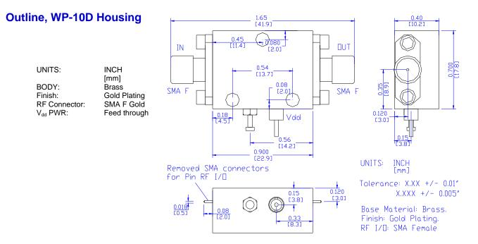
For the pin type input and output application, remove the input and output SMA connectors.
