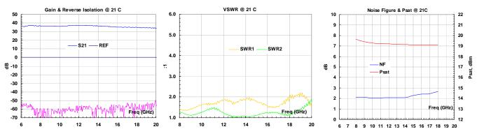
\*The measured noise figure includes the input SMA connector loss. The noise figure shall be around 0.1 dB lower without Input SMA connector.
