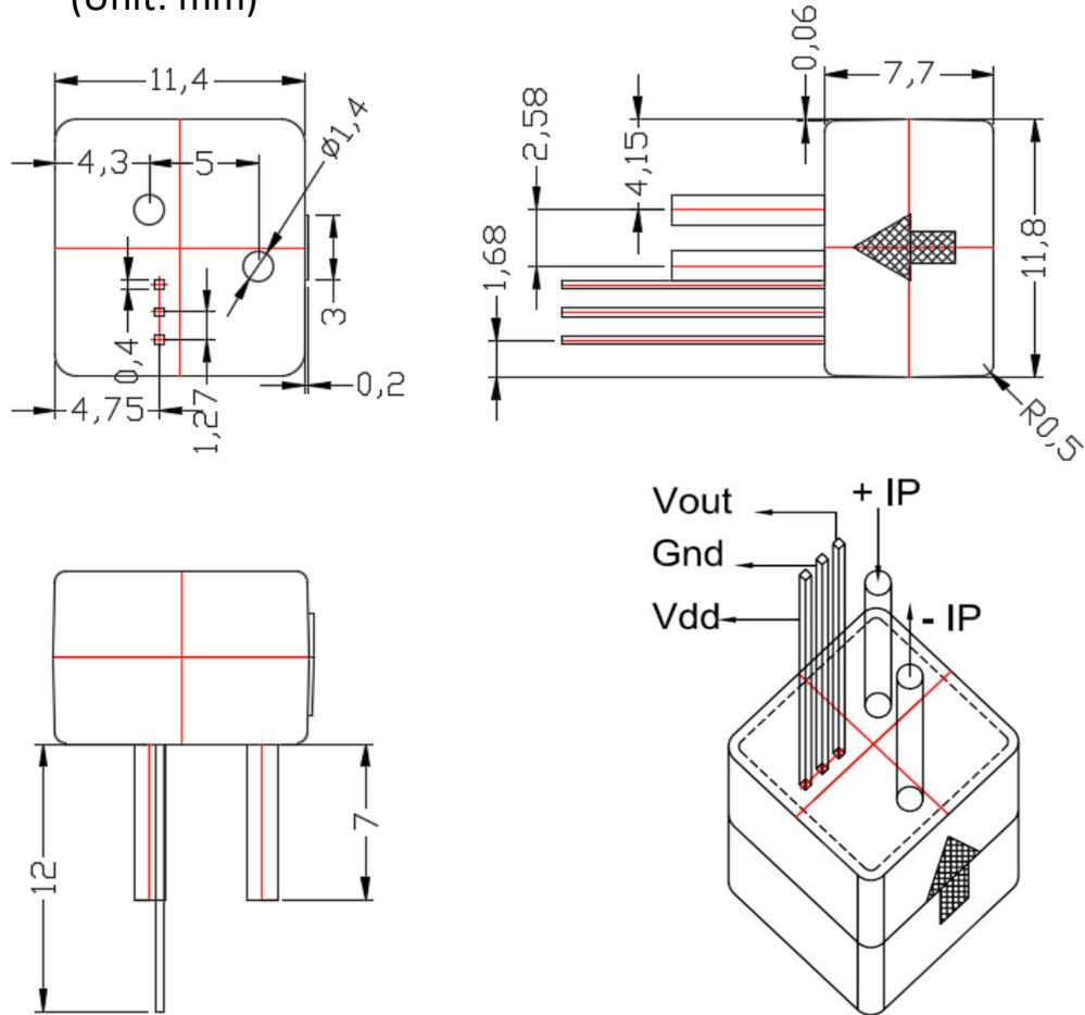
PCB Layout Reference View( Top View)
