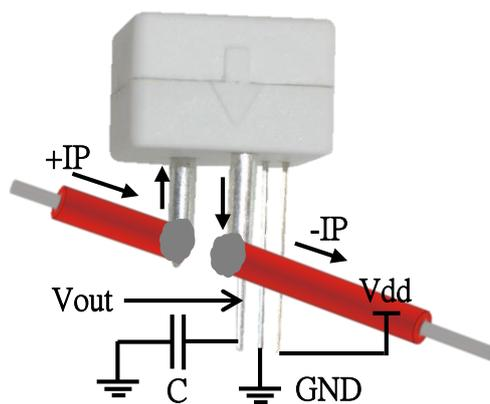
Capacitor **C**(0.01uF~0.1uF) is recommend to be connected between Vout and GND to reduce output noise.
