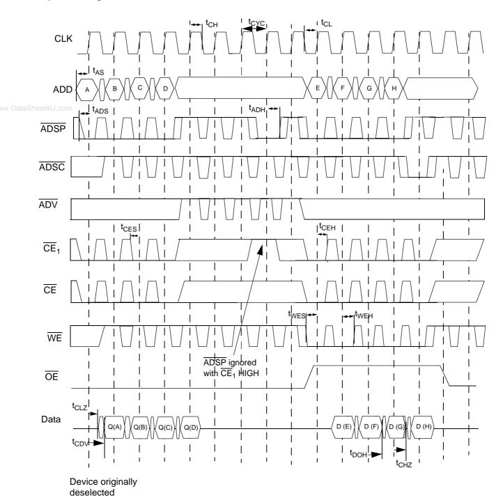
$\overline{\text{CE}}$  is the combination of  $\text{CE}_2$  and  $\overline{\text{CE}}_3$ . All chip selects need to be active in order to select the device. RAx stands for Read Address X, WAx stands for Write Address X, Dx stands for Data-in X, Qx stands for Data-out X.
