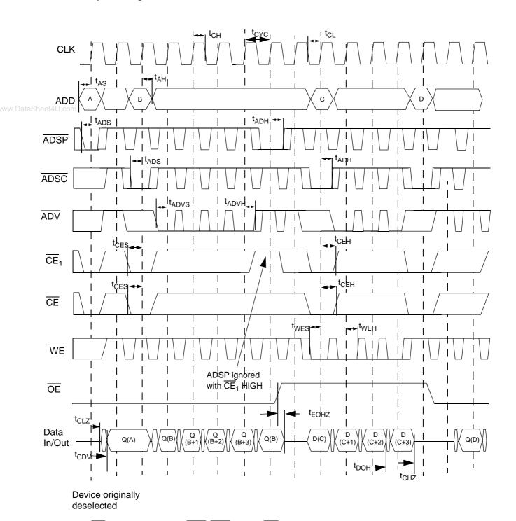
$\overline{\text{WE}}$  is the combination of  $\overline{\text{BWE}}$ ,  $\overline{\text{BWS}}_{\text{[1:0]}}$ , and  $\overline{\text{GW}}$  to define a write cycle (see Write Cycle Descriptions table)  $\overline{\text{CE}}$  is the combination of  $\overline{\text{CE}}_2$  and  $\overline{\text{CE}}_3$ . All chip selects need to be active in order to select the device. RAx stands for Read Address X, WAx stands for Write Address X, Dx stands for Data-in X, Qx stands for Data-out X.
