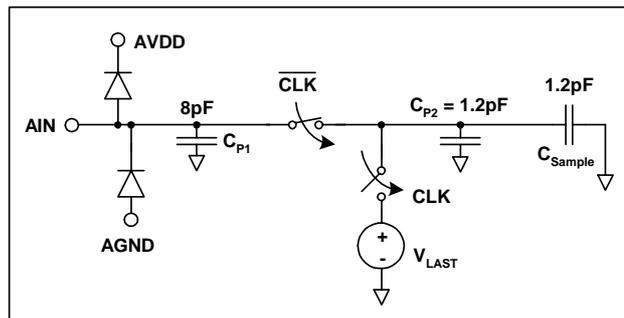
Figure 20 Equivalent Circuit for Analogue Input Pin AIN
