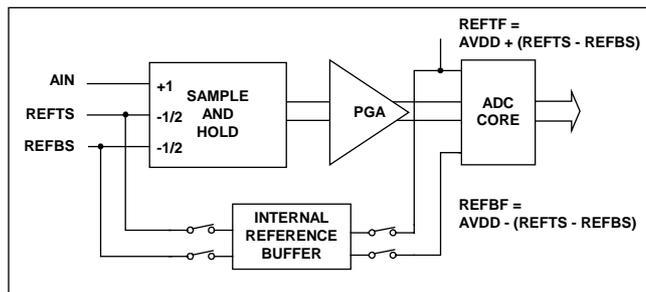
Figure 13 ADC Reference Generation in Top/Bottom Mode
