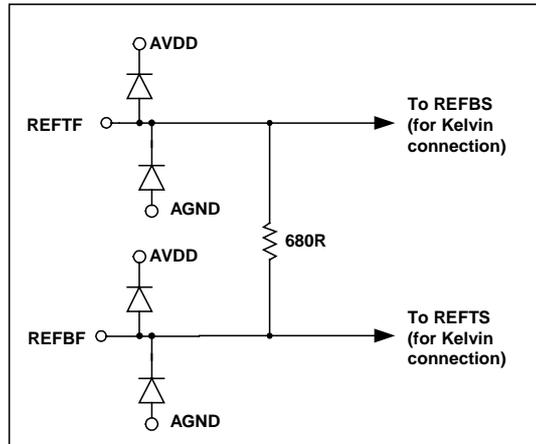
**Figure 26 Equivalent Circuit of REFTF and REFBF Inputs**
