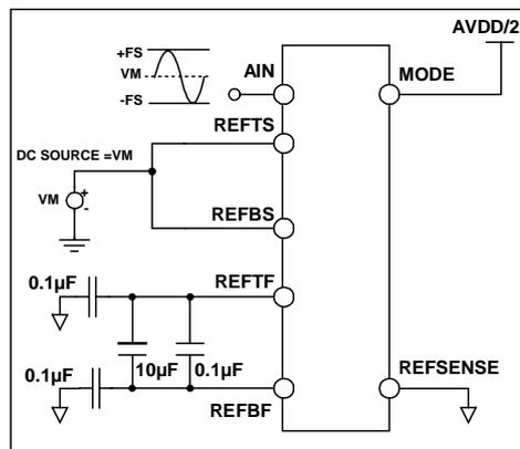
Figure 12 Centre Span Mode, 2V Reference Span
