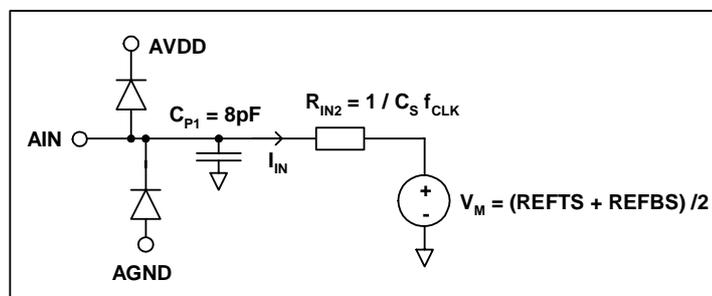
Figure 21 Equivalent Circuit for the AIN Switched Capacitor Input
