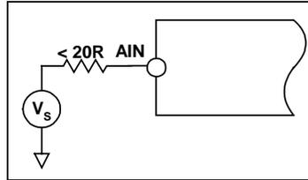
**Figure 22 Damping Source Ringing Using a Small Resistor**
