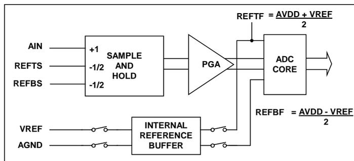
Figure 10 ADC Reference Generation in Differential Mode
