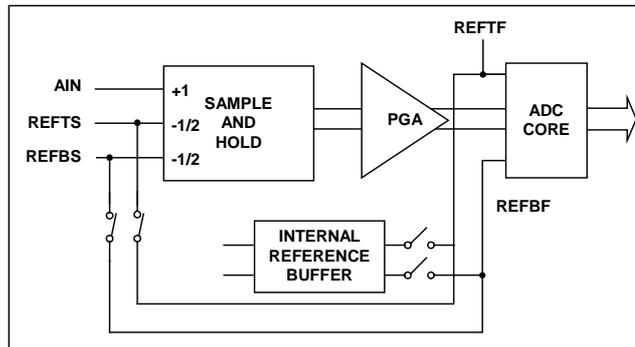
Figure 7 ADC Reference Generation in Full External Mode
