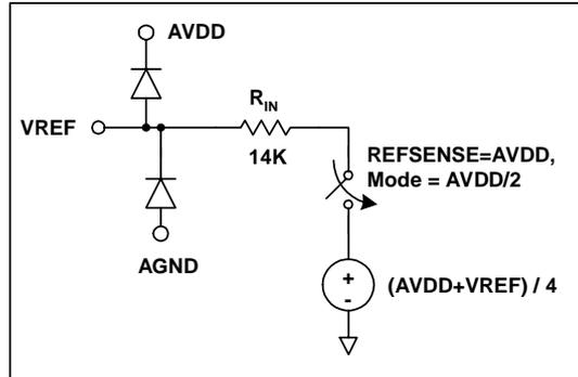
Figure 24 Equivalent Circuit of VREF
