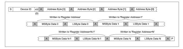
Figure 75 Multiple Register Write to Specified Address using Auto-increment
