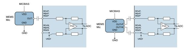
Figure 84 Single-Ended and Differential Analogue Microphone Connections
