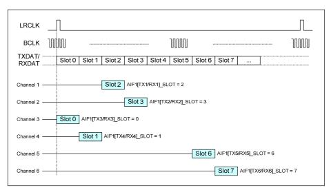
Figure 50 DSP Mode B Example
