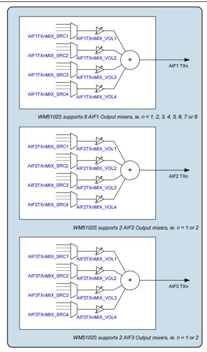
Figure 25 Digital Core AIF Outputs
