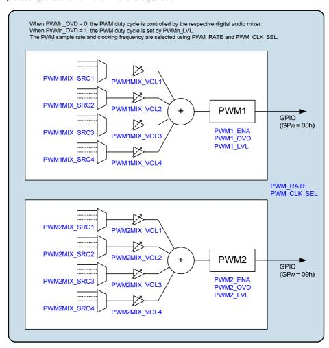
Figure 37 Digital Core Pulse Width Modulation (PWM) Generator
