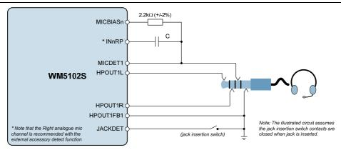
Figure 91 External Accessory Detection
