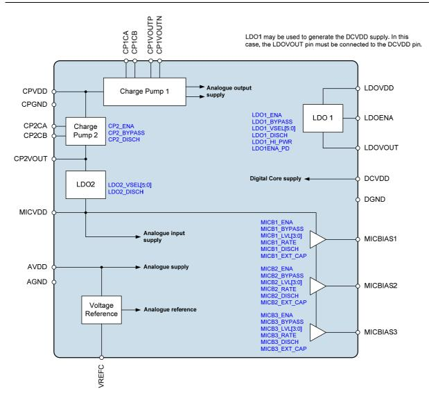
Figure 81 Charge Pumps and Regulators
