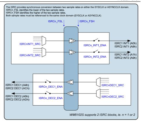
Figure 41 Isochronous Sample Rate Converters (ISRCs)
