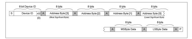
Figure 73 Single Register Write to Specified Address
