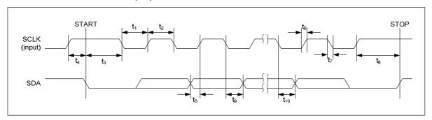
Figure 9 Control Interface Timing - 2-wire (I2C) Control Mode
