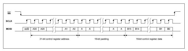
Figure 78 Control Interface 4-wire (SPI) Register Write
