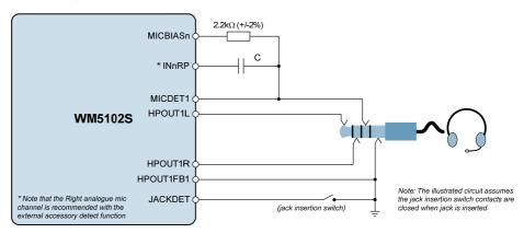
Figure 61 Jack Detect and External Accessory Connections
