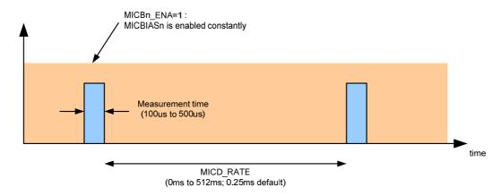
Figure 65 Microphone and Accessory Detect Timing
