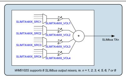
Figure 27 Digital Core SLIMbus Outputs
