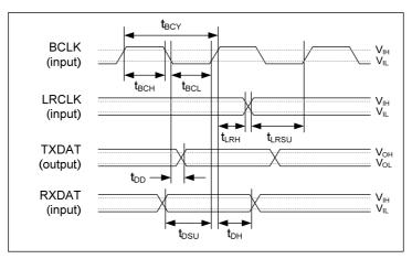
Figure 7 Audio Interface Timing - Slave Mode
