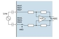
Figure 18 Single-Ended Line Input
