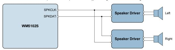
Figure 60 Digital Speaker (PDM) Connection
