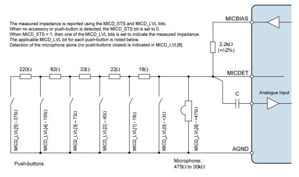
Figure 92 External Accessory Detect Connection
