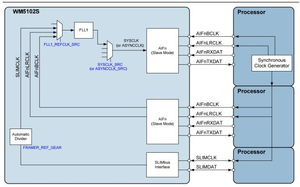
Figure 99 AIF Slave Mode, using another Interface as Reference
