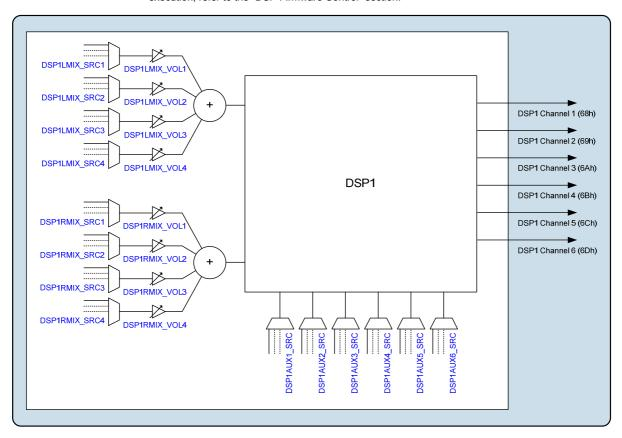
Figure 33 Digital Core DSP Block
