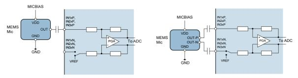
Figure 16 Single-Ended MEMS Input
