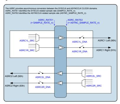
Figure 40 Asynchronous Sample Rate Converters (ASRCs)
