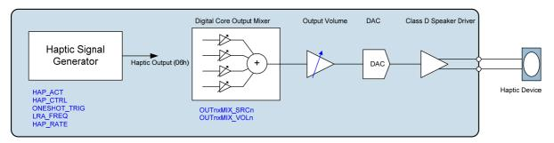
Figure 36 Digital Core Haptic Signal Generator
