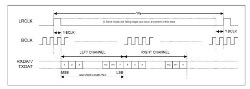
Figure 45 DSP Mode A Data Format
