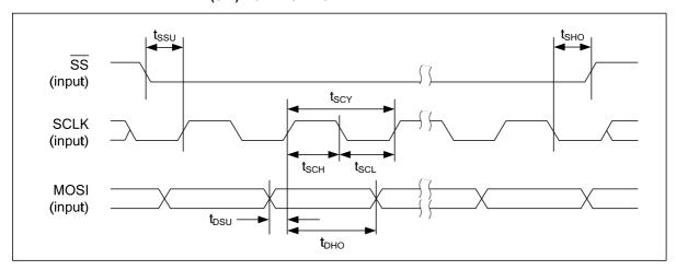
Figure 10 Control Interface Timing - 4-wire (SPI) Control Mode (Write Cycle)
