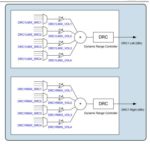
Figure 30 Dynamic Range Control (DRC) Block
