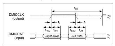
Figure 3 Digital Microphone Interface Timing
