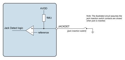
Figure 62 Jack Detect Comparator
