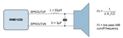
Figure 89 Class D Output Filter Components
