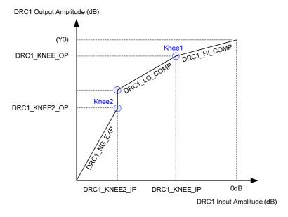
Figure 31 DRC Response Characteristic
