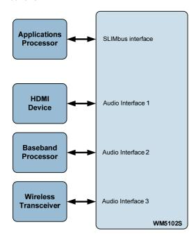
Figure 42 Typical AIF Connections
