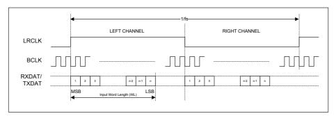
Figure 48 Left Justified Data Format (assuming n-bit word length)
