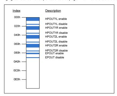
Figure 80 Write Sequencer Memory
