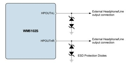
Figure 87 ESD Diode Configuration for External Output Connections
