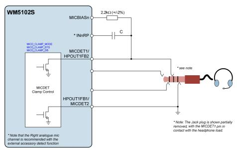
Figure 63 MICDET Clamp circuit
