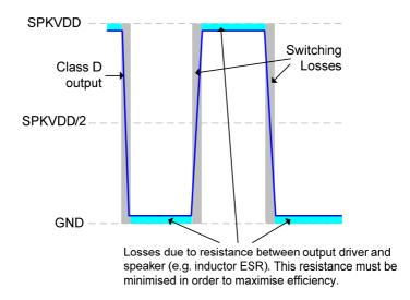
Figure 88 Speaker Connection Losses
