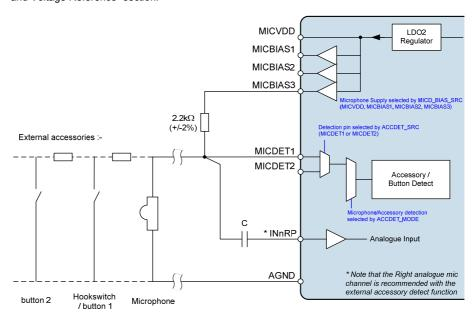
Figure 64 Microphone and Accessory Detect Interface
