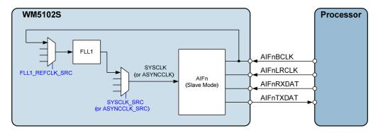
Figure 96 AIF Slave Mode, using BCLK and FLL as Reference
