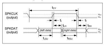
Figure 4 Digital Speaker (PDM) Interface Timing - Mode A
