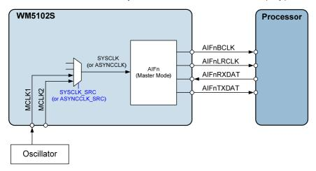
Figure 93 AIF Master Mode, using MCLK as Reference
