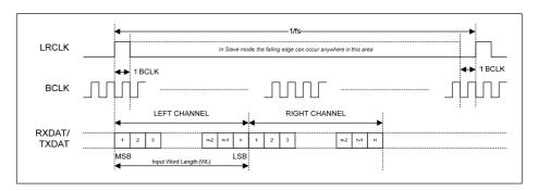
Figure 46 DSP Mode B Data Format
