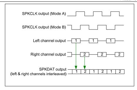
Figure 59 Digital Speaker (PDM) Interface Timing
