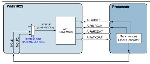
Figure 97 AIF Slave Mode, using MCLK as Reference
