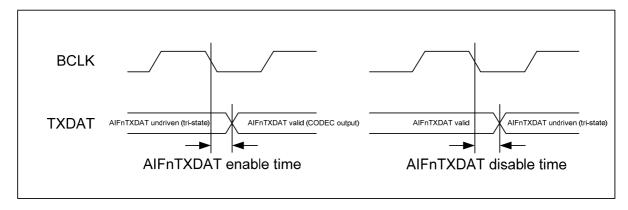
Figure 8 Audio Interface Timing - TDM Mode
