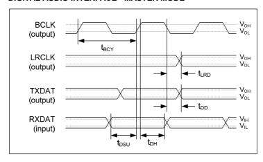
Figure 6 Audio Interface Timing - Master Mode
