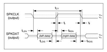
Figure 5 Digital Speaker (PDM) Interface Timing - Mode B
