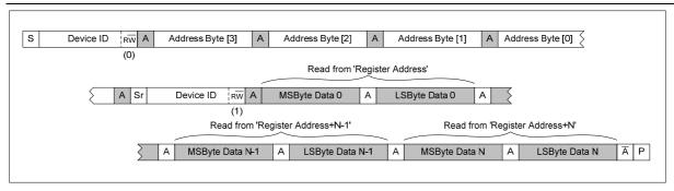
Figure 76 Multiple Register Read from Specified Address using Auto-increment
