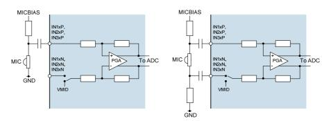
Figure 83 Single-Ended and Differential Analogue Microphone Connections
