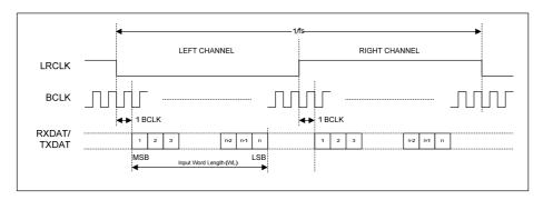
Figure 47 I2S Data Format (assuming n-bit word length)
