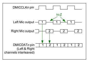
Figure 21 Digital Microphone Interface Timing
