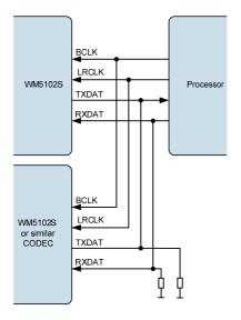
Figure 55 TDM with Processor as Master
