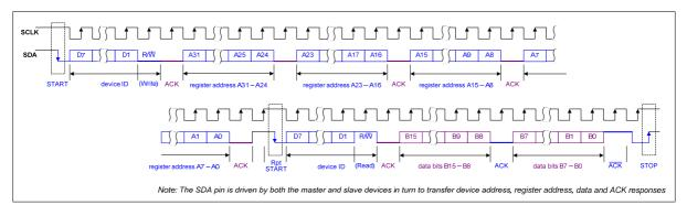
Figure 72 Control Interface 2-wire (I2C) Register Read
