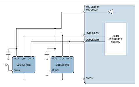
Figure 20 Digital Microphone Input
