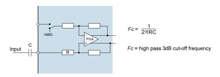
Figure 82 Audio Input Path DC Blocking Capacitor
