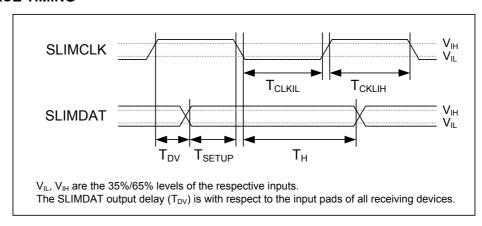
Figure 12 SLIMbus Interface Timing
