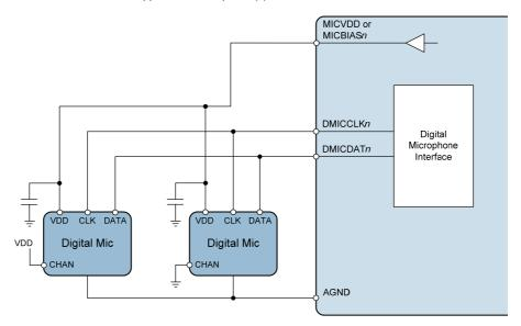
Figure 85 Digital Microphone Connection
