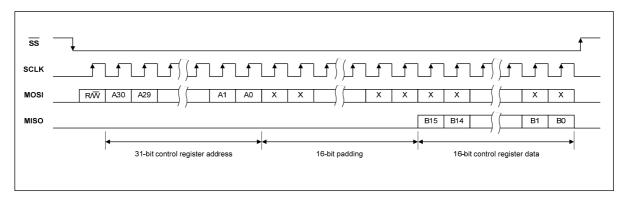
Figure 79 Control Interface 4-wire (SPI) Register Read
