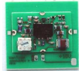
Fig. 3 Assembled preamp
