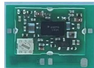
Fig. 3 Assembled preamp
