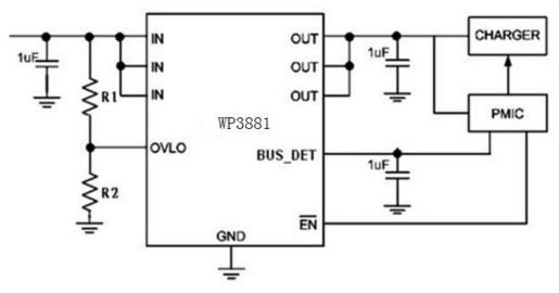
Note: R1 and R2 are only required for adjustable OVLO; Otherwise OVLO is connected to GND.
