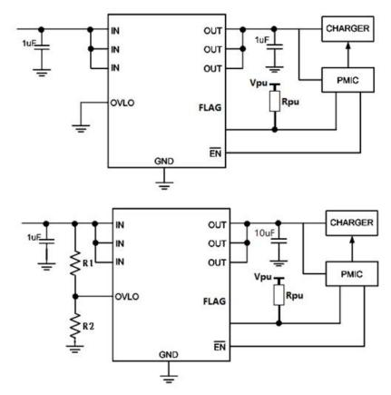
Note1: R1 and R2 are only required for adjustable OVLO; Otherwise OVLO is connected to GND.
