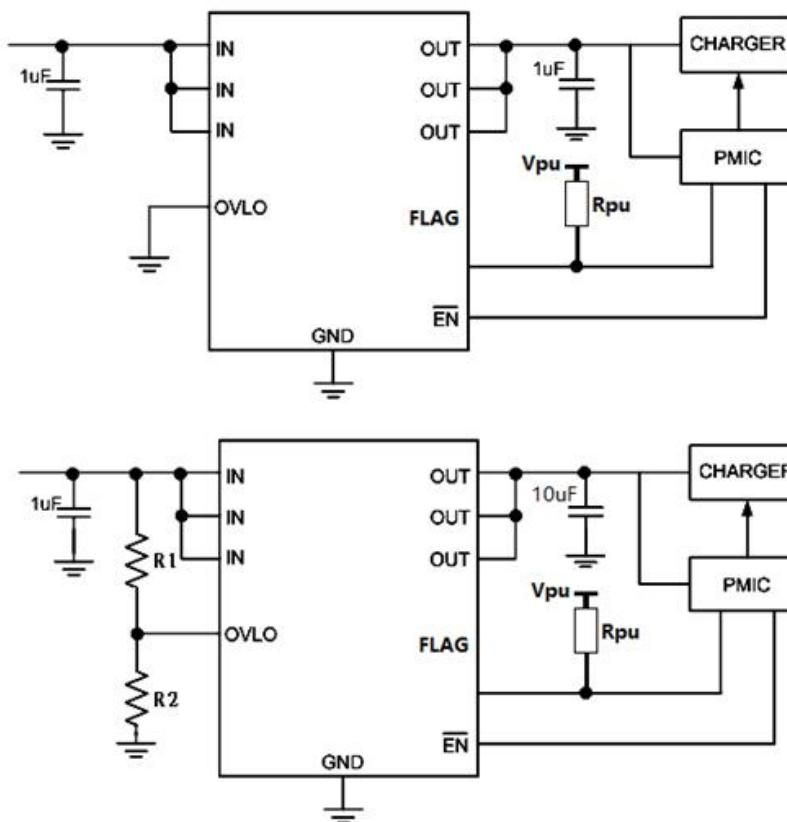
Note1: R1 and R2 are only required for adjustable OVLO; Otherwise OVLO is connected to GND.
