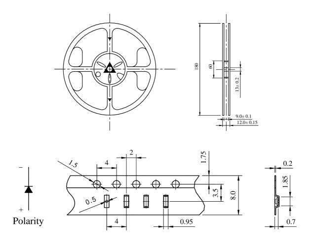
Reel Lead Min.60mm No LEDs
