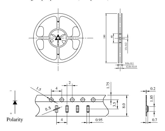
Reel Lead Min.60mm No LEDs
