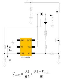
R1: The resistor connected from PRT to AUX.
