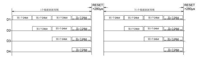
Note: The data of D1 is sent by MCU, and D2, D3, D4 through pixel internal reshaping amplification to transmit.
