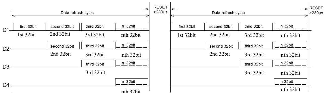
Note: D1 is the data sent by the MCU, and D2, D3, and D4 are the data automatically shaped and forwarded by the cascade circuit.
