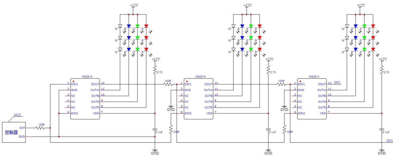
24V power supply application reference circuit (each channel with 6 LEDs):
