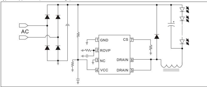
Attention: A 22pF capacitor can be parallel with Rovp and a resistor can be parallel with the Vcc capacitor.
