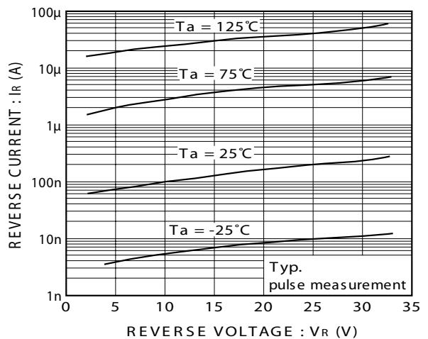
Fig. 2 Reverse characteristics
