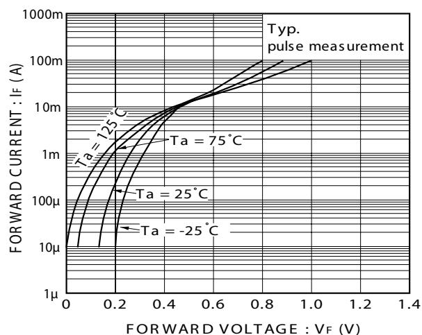
Fig. 1 Forward characteristics
