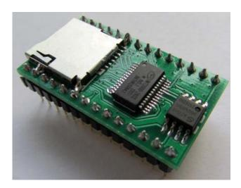
WT2000M03 is MP3 module, with folder classify, specified file name play and specified index sequence play. According file name to record in specified file or according index sequence to record and play. Support SPI-Flash, TF card and U disk.
