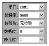
Serial port: COM1 Baud rate: 9600 Check bit: Don't check Datacode: 8, End code: 1
