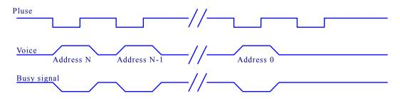
**Note:** Negative trigger pulse. Trigger with a button to play a sound. A pulse plays a piece, the next pulse plays the last piece. No longer trigger forward when the front voice is over. Repeat the operation, can only play to the last.
