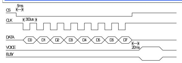
**Description:** WT588D-U voice module begins to send data signals after current is switched on and wairt 17ms.
