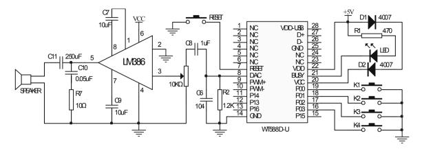
**Note:** DAC output port together with the ground, which connect with a 1.2K resistor and capacitor 104. when use DAC output way, and then the audio signal re-entering amplifier part, as circuit diagram of R2, R6 shown.
