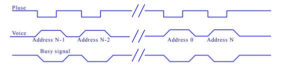
**Note:** Negative trigger pulse. Trigger with a button to play a sound. A pulse plays a piece, the next pulse plays the last piece. Repeat the operation. It will start again from the last piece when the front shows off. Loop continuously.
