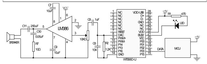
**Note:** DAC output port together with the land, which connect with a 1.2K resistor and capacitor 104. when use DAC output way, and then the audio signal re-entering amplifier part, as circuit diagram of R2, R6 shown.
