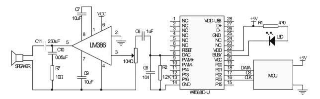
Note: DAC output port together with the ground, which connect with a 1.2K resistor and capacitor 104.
