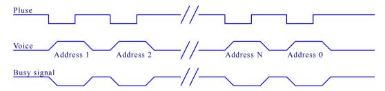
**Note:** Negative trigger pulse. Trigger with a button to play a sound. A pulse plays a piece , the next pulse plays the next piece. Repeat the operation. It will start again from the first piece when the last shows off. Loop continuously.
