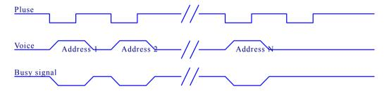
**Note:** Negative trigger pulse. Trigger with a button to play a sound. A pulse plays a piece, the next pulse plays the next piece. It doesn't stop until the last piece is finished. Repeat the same operation. Can only play to the last.
