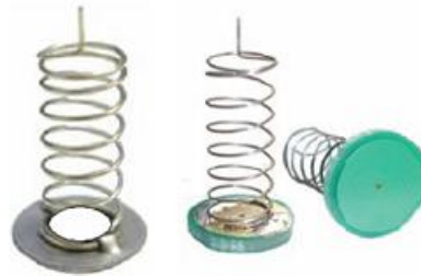
Figure 3: capacitance sensor for metal spring (key sense element)
