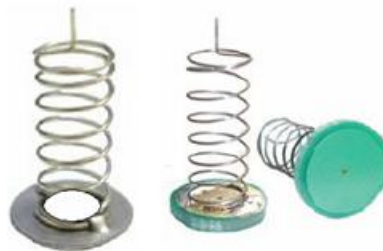
Figure 4: capacitance sensor made by metal spring (key sense element)
