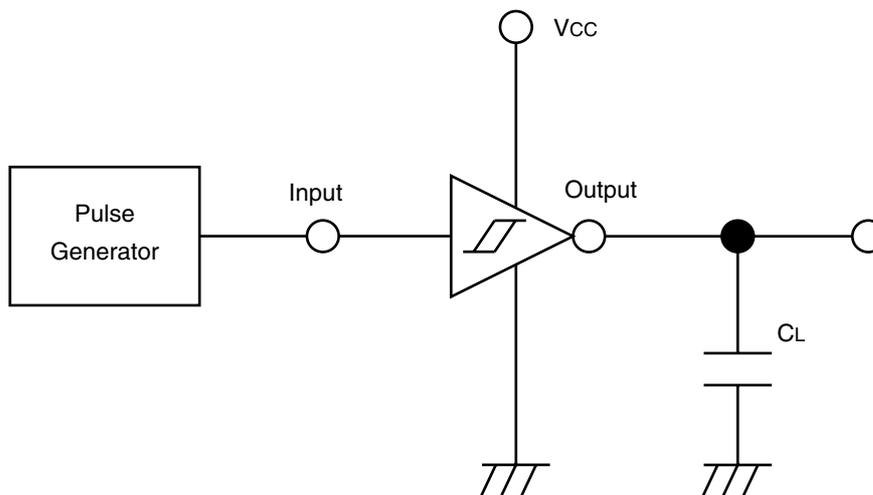
Note: open output when measuring supply current
