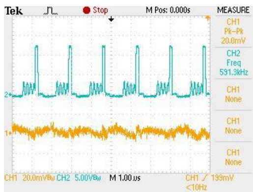
STEADY STATE OPERATION (VIN=12V, VOUT=1.2V, IOUT=100mA)
