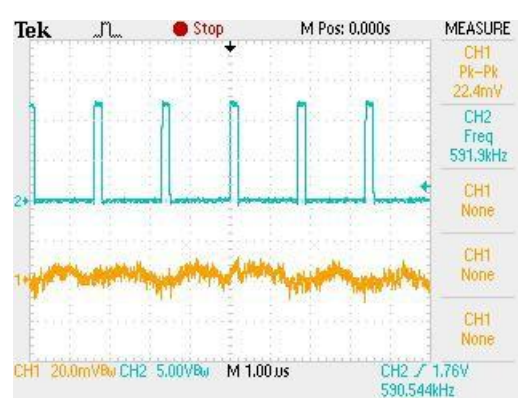
STEADY STATE OPERATION (VIN=12V, VOUT=1.2V, IOUT=1000mA)
