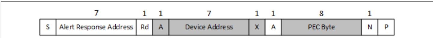
Figure 30 A 7-bit-Addressable Device responds to an ARA with PEC
