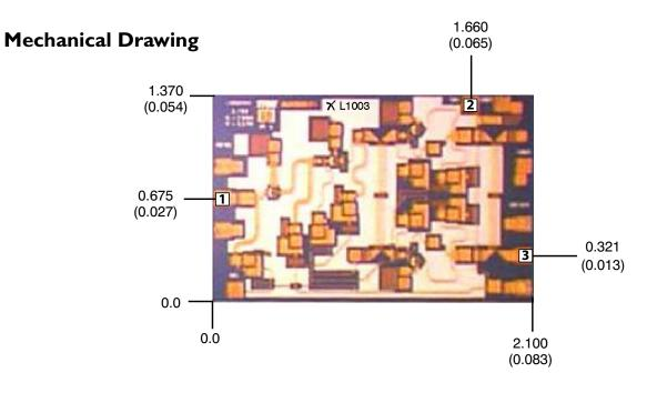
Units: millimeters (inches) Bond pad dimensions are shown to center of bond pad. Thickness: 0.110 +/- 0.010 (0.0043 +/- 0.0004), Backside is ground, Bond Pad/Backside Metallization: Gold All Bond Pads are 0.100 x 0.100 (0.004 x 0.004).
