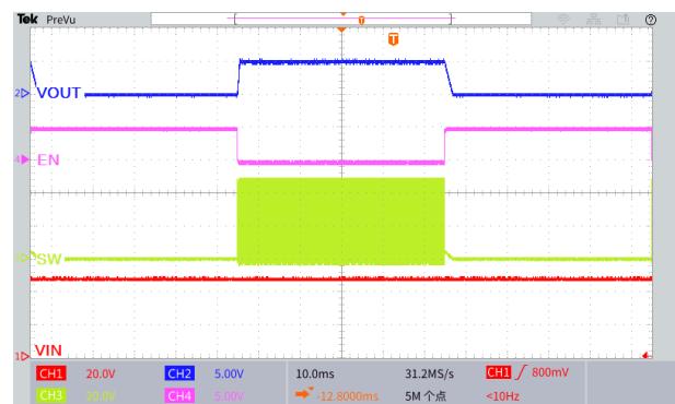
Figure39. Start or Shutdown Using EN Pin ( V_{IN}=48V , V_{OUT}=5.0V , I_{OUT}=0.5A )
