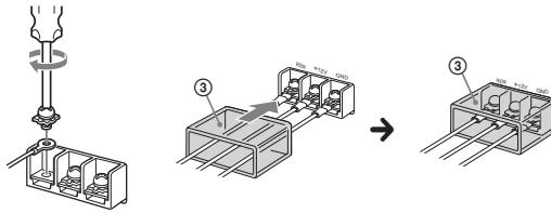
**Pass the wires through the cap, connect the wires, then cover the terminals with the cap.**
