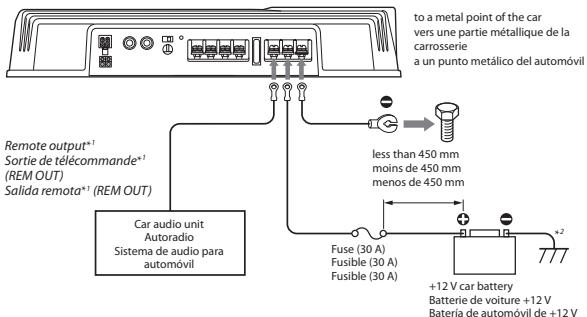
\*<sup>1</sup> If you have the factory original or some other car audio unit without a remote output for the amplifier, connect the remote input terminal (REMOTE) to the accessory power supply. In High level input connection, car audio unit can also be activated without need for REMOTE connection. However, this function is not guaranteed for all car audio units.
