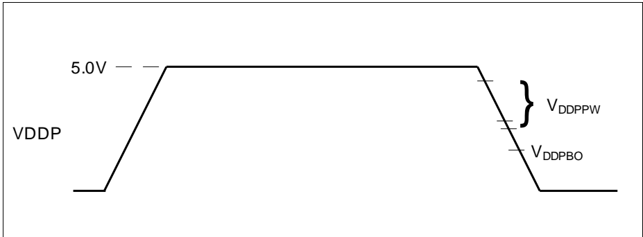
Figure 14 Supply Threshold Parameters
