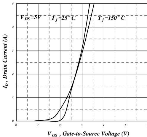
**Fig 11. Transfer Characteristics**
