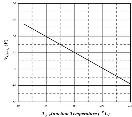
**Fig 6. Gate Threshold Voltage v.s. Junction Temperature**
