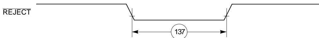
Figure 63. CAM Interface \overline{\text{REJECT}} Timing Diagram
