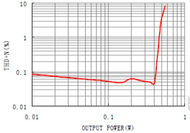
THD+N vs OutputPower VDD=2.5V, RL=8Ω, and f=1KHz
