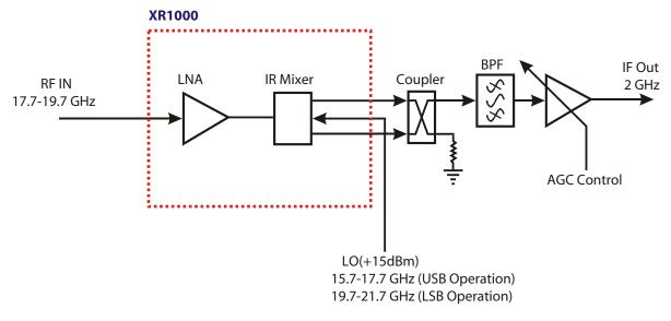
Mimix Broadband MMIC-based 17.0-27.0 GHz Receiver Block Diagram (Changing LO and IF frequencies as required allows design to operate as high as 27 GHz)
