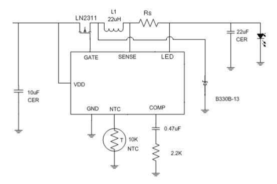
Note: Rs set the LED current resistor, the LED current  $I_{LED} = \frac{100mV}{R_s}$ , NTC pin can directly connect to ground.
