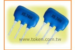
with 2 trap frequencies. Recommended for Multi standard set. Features with good performance of attenuation and space saving with 3-terminal type. The characteristic of a three-terminal ceramic trap equals two two-terminal ceramic traps. Three-terminal ceramic trap has a monolith structure formed from 2 ceramic resonators.
