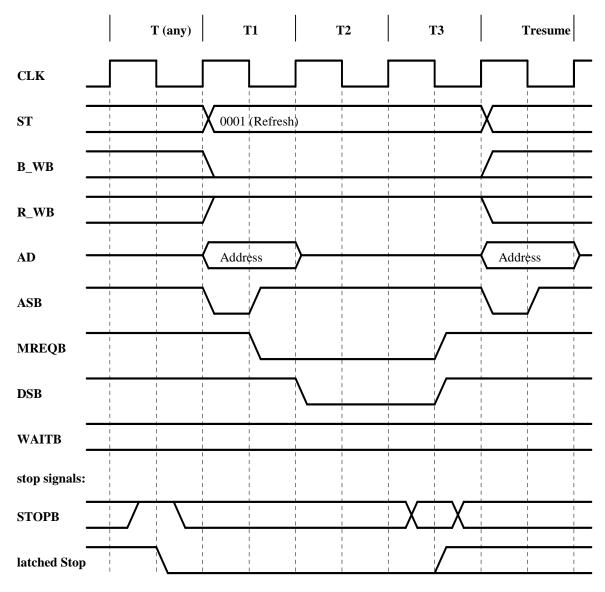
The figure below shows the de-assertion of the Stop Request:
