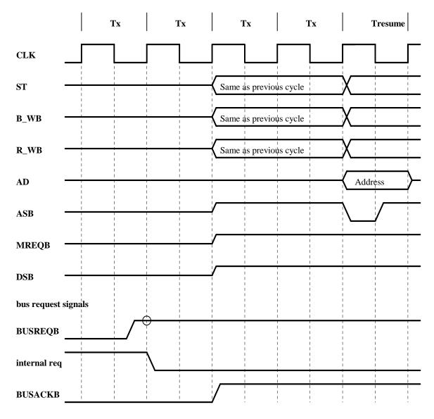
The figure below shows the sampling of Bus Request and the exit from the Bus Acknowledge state:
