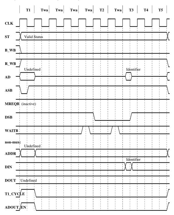
Note that the Wait Request input is sampled twice during this bus transaction, once before the Data Strobe is activated and once while Data Strobe is active. Memory write bus transactions follow immediately, to save the program status.
