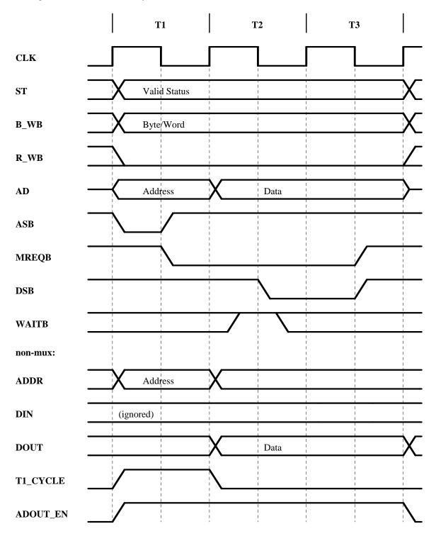
Note that for memory write cycles the DSB signal is delayed by one-half clock cycle to guarantee that the data bus is valid prior to the leading edge of DSB.
