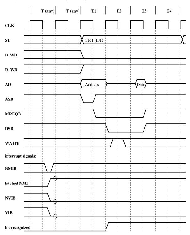
Note that the aborted IF1 transaction is always 4 clock cycles (plus Wait states) long in this design. The Z8000 documentation indicates that this aborted IF1 transaction may be from 3 to 7 cycles (plus Wait states) long. An interrupt acknowledge transaction follows immediately after this aborted IF1 transaction.
