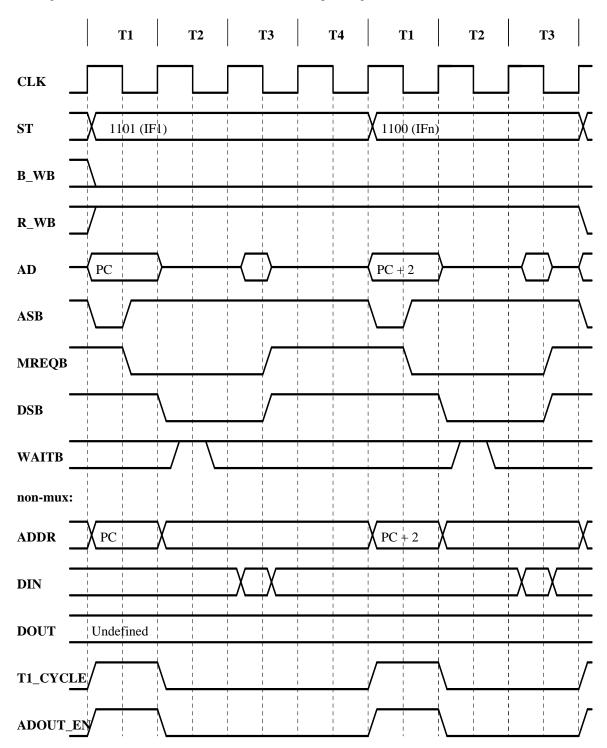
The instruction fetched during the IF1 bus transaction is pushed as the identifier for this trap. The word fetched during the IFn bus transaction is ignored. The Program Counter does not increment beyond PC + 2, and this is the value pushed on the stack.
