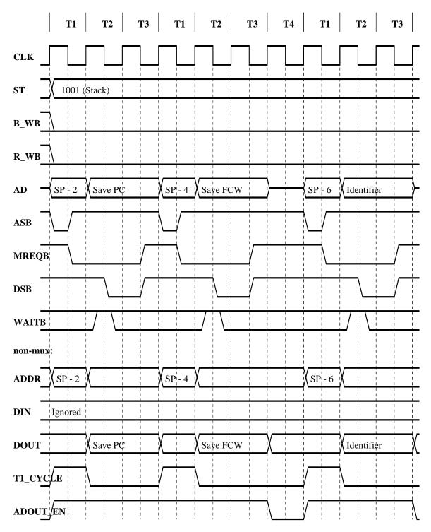
The figure below shows the status saving sequence common to both interrupts and traps:
