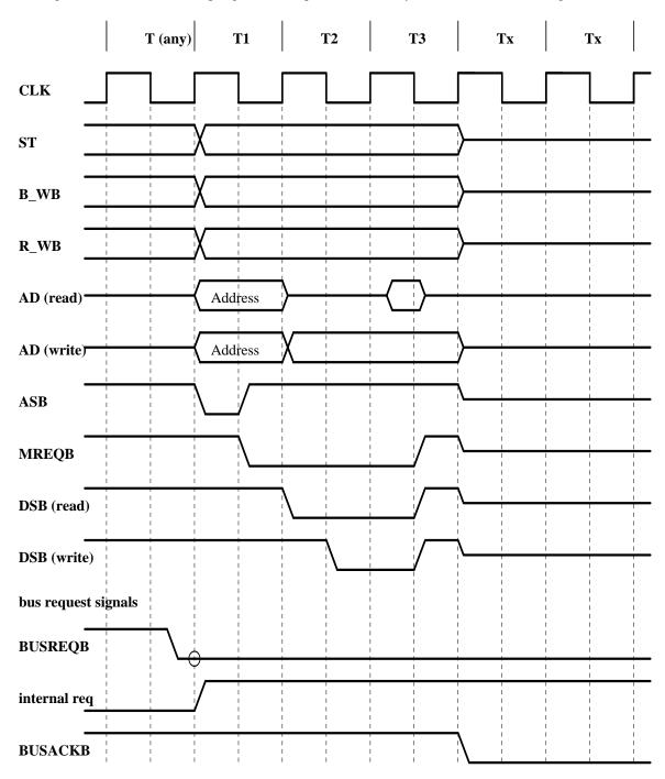
The figure below shows the sampling of Bus Request and the entry into the Bus Acknowledge state:
