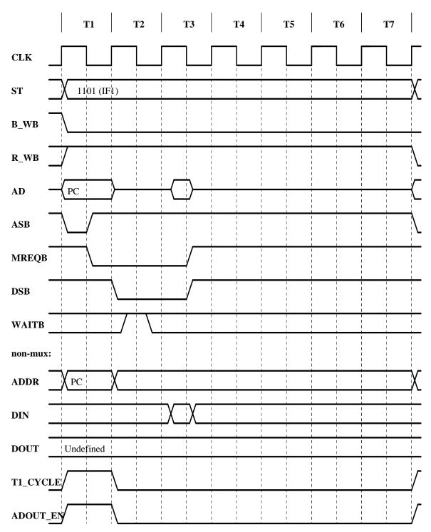
This is the case used by the System Call instruction, plus a number of illegal instructions. The timing for all of the different cases of a trap are identical, and only the signals during cycles 4-7 of the sequences are different.
