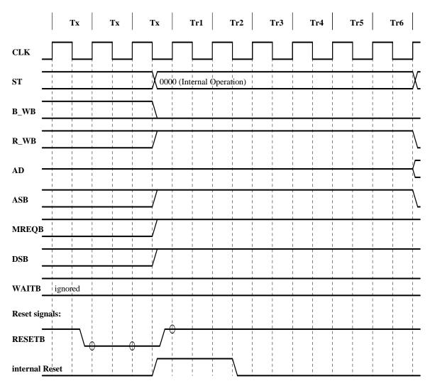
The figure below shows the Reset timing and reset sequence:
