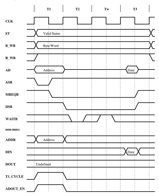
The figure below shows a memory write bus transaction, with one wait state:
