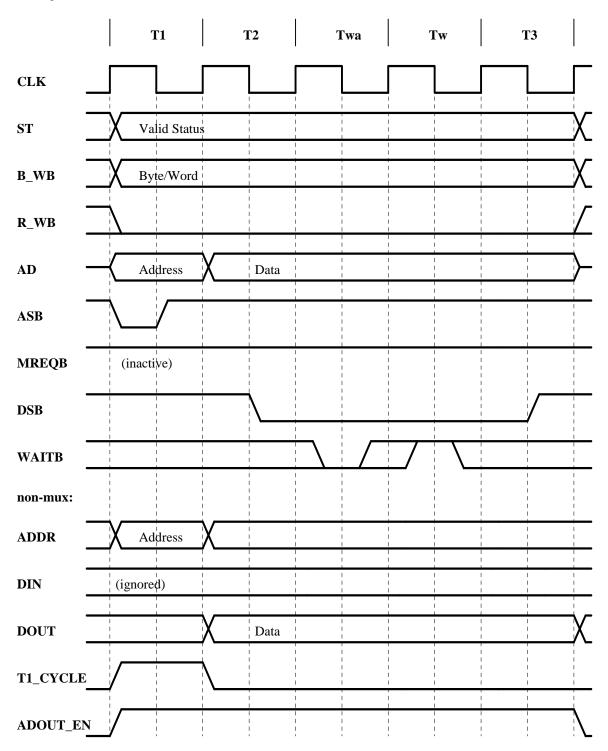
The figure below shows an internal operation bus transaction:
