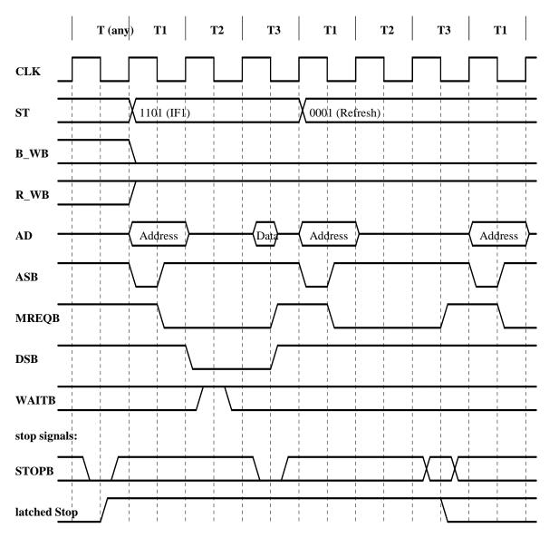
The figure below shows how the Stop Request is sampled:
