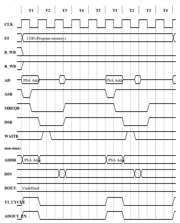
The figure below shows the Program Status Area fetch sequence common to reset, traps and interrupts:
