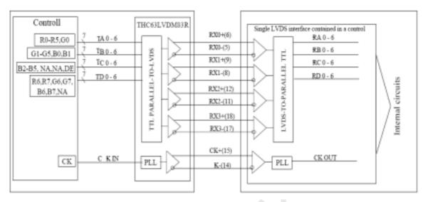
(2) 8bit Mode LVDS\_SET=L (20 pin=GND or OPEN)
