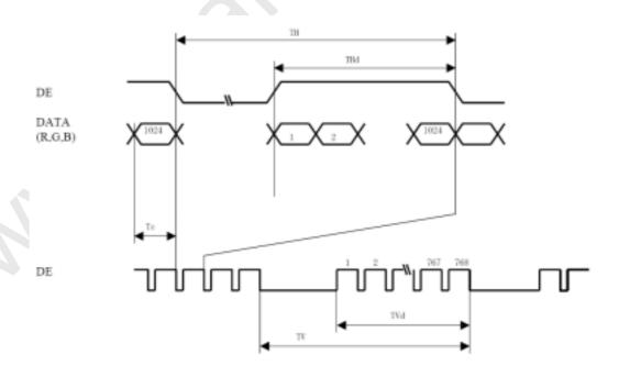
7-2 Input Data Signals and Display Position on the screen
