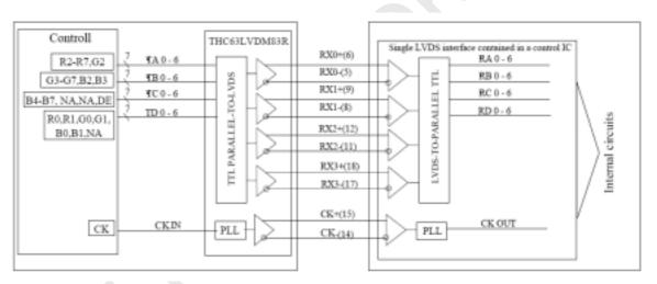
(3) 6bit Mode LVDS\_SET=L (20 pin=GND or OPEN)
