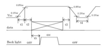
Power sequence for Backlight is not especially specified, however it is recommended to consider some timing difference between LVDS input and Backlight input as shown above.
