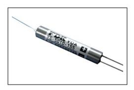
The YS-5010 is a variable optical attenuator applying the Faraday effect of magneto-optical crystals. The attenuation levels can be adjusted continuously by current control. Due to the exclusion of any moving parts, it has attained a high reliability and rapid response.
