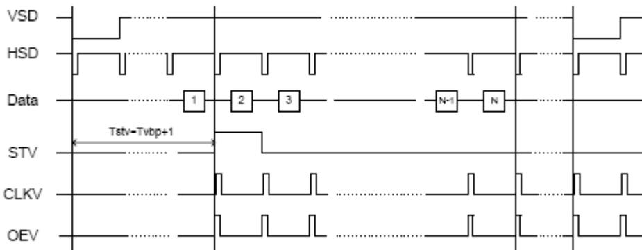
Vertical timing diagram HV (Cascade)
