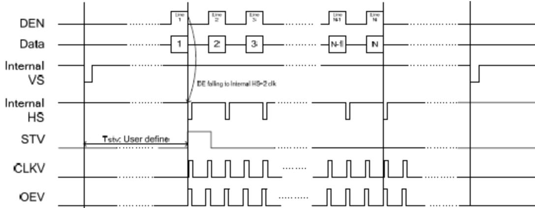
**Vertical timing diagram DE (Dual gate)**
