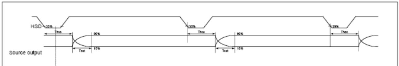
Source output timing diagram (Cascade)
