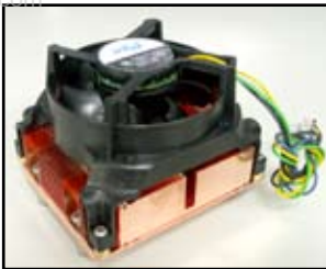
CPU heatsink (top view)
