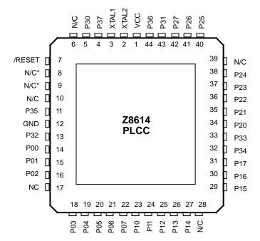
Note: Pins 8 and 9 actually are connected to the chip, although used only for testing. These pins must be used as floaters by the customer.
