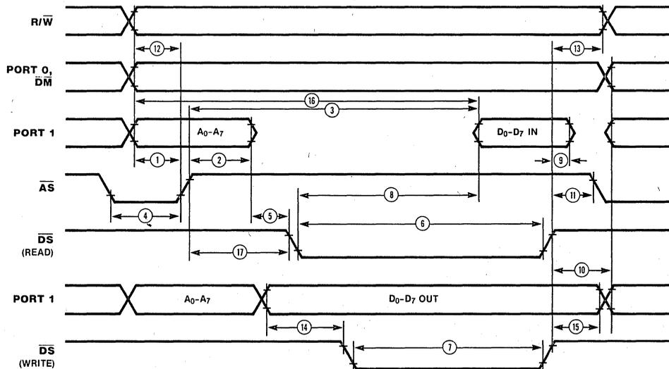
Figure 15. External I/O or Memory Read/Write Timing
