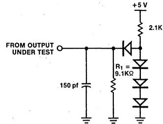
Figure 14. Test Load 1
