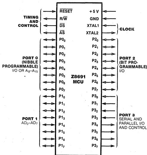
Figure 1. Pin Functions
