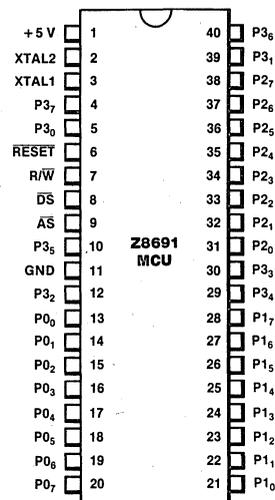
Figure 2a. 40-pin Dual-In-Line Package (DIP), Pin Assignments
