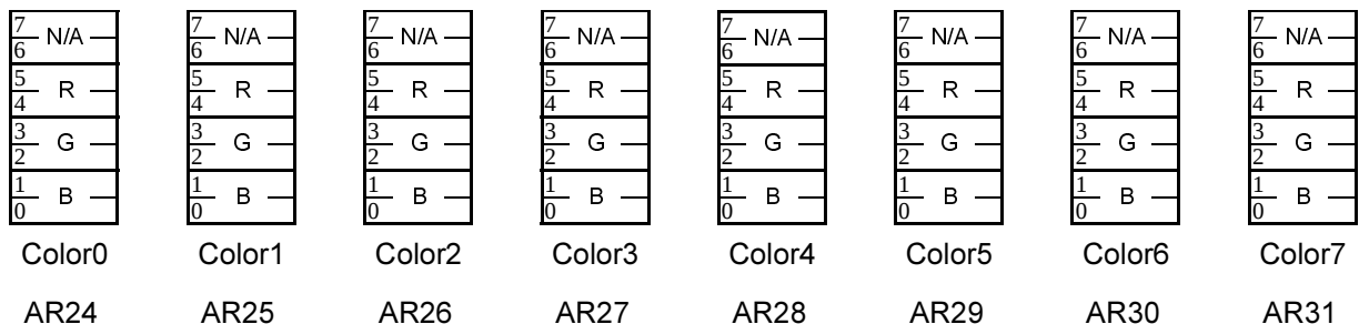
Figure 24 Programmable Palette Control at AR Register
