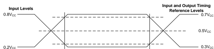
Figure 8.3 AC Measurement I/O Waveform
